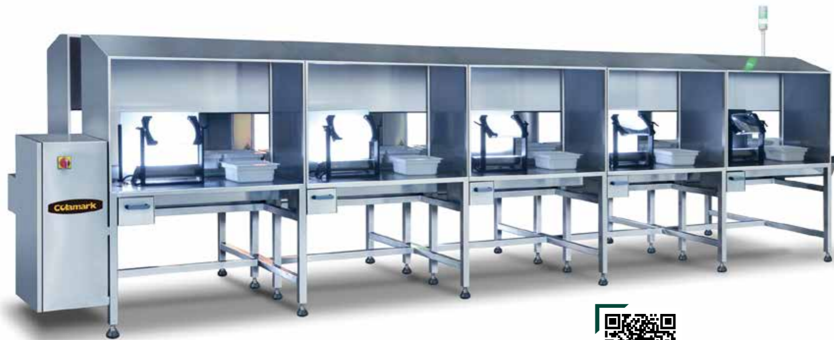
10 station semi-automatic lamp inspection system
