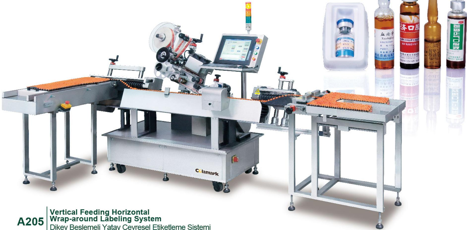
**A205** | **Vertical Feeding Horizontal Wrap-around Labeling System**
