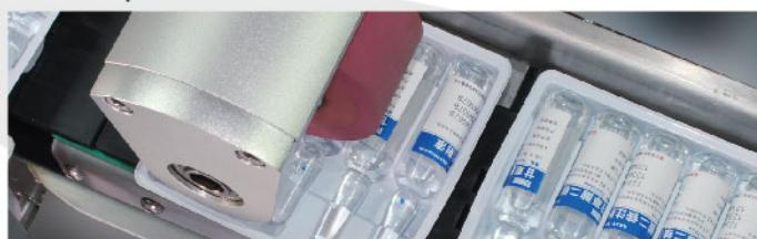
RH1 is specifically designed for inserting labeled round bottles horizontally into the base tray for subsequent cartoning. Using a uniquely designed buffering tank, an "S" shaped inserting path, and a servo controlled driving wheel, the RH1 operates smoothly at very high speed, and achieve seamless integration with the Colamark horizontal round bottle labeling systems.
