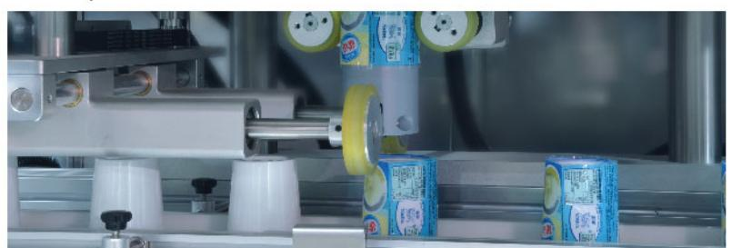
An ideal system for inserting sleeve labels on to bottles or other types of packaging containers at high speed. Patented negative pressure film buffering mechanism and servo controlled satellite label cutting blades ensure the smooth and stable processes of label feeding, cutting, and ejection.
